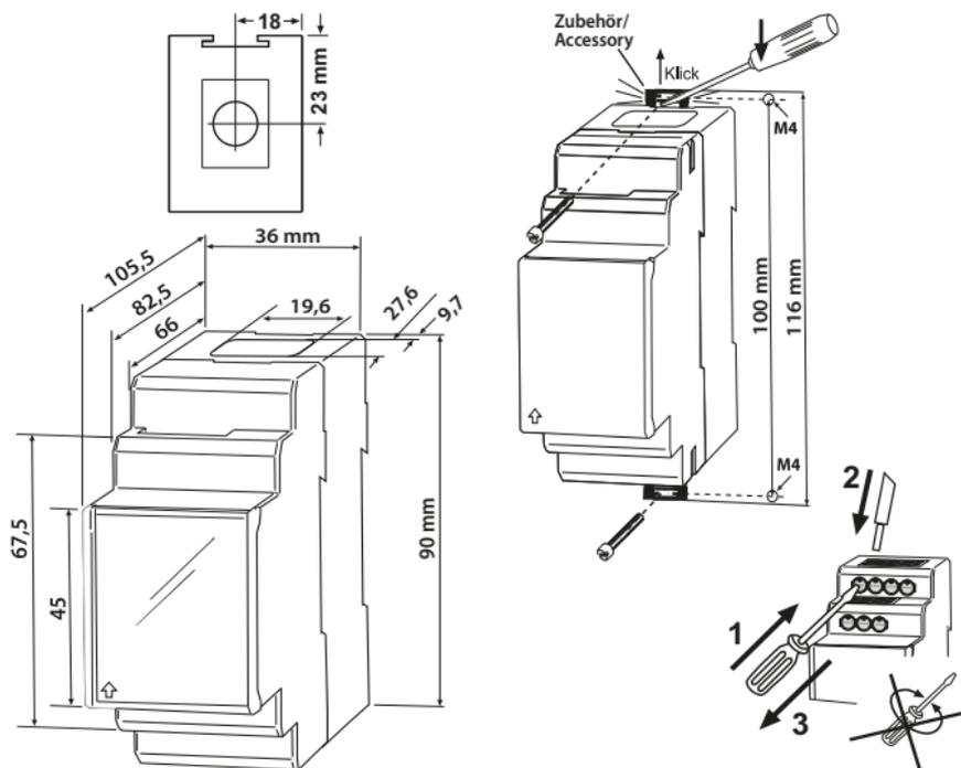
The front plate cover is easy to open at the lower part marked by an arrow.
