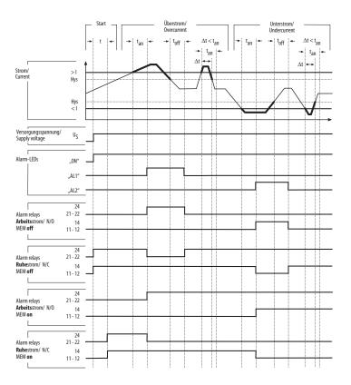
t = Starting delay,  $t_{an}$  = Response time,  $t_{off}$  = Delay on release
