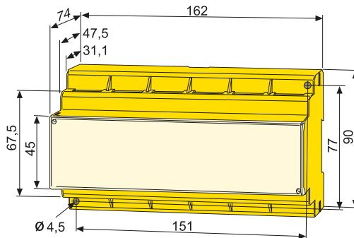
**Dimension diagramm** (dimensions in mm)
