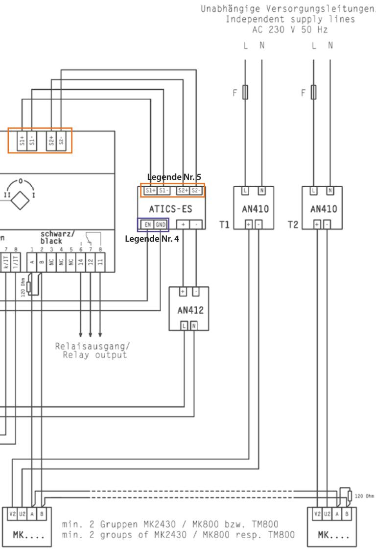
The ATICS-ES energy storage device is only allowed to be installed in a switch cabinet with a cover.
