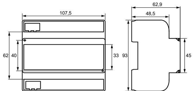
Dimension diagram (in mm)
